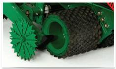
A forward metering wheel helps measure and cut sod accurately.
