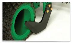
Durable cutting blade is easily adjustable down to a depth of 2  $\frac{1}{2}$ " and can change angles to match soil and blade conditions.
