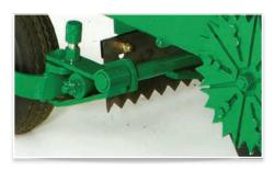
Automatic sod cutoff provides precise cutting of sod strips from one to six feet long.
