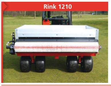
The Rink 1210 has low sides, for easy refilling and ensures the operator has a good rear view.
