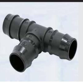
The DB range can be confidently installed without clamps when matched to quality low pressure poly tubing with corresponding dimensions (refer to the tubing manufacturer for confirmation of suitability or test under field conditions). Operating pressures should not exceed 300 kPa.
