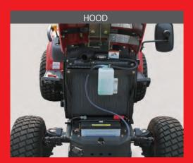
An extremely wide-opening hood provides good serviceability to the engine, air filter, and electrical components.
