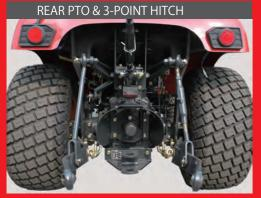
Combined with the rear PTO and SAE category-1 three-point hitch, a variety of implements and attachments can be fitted according to the type of works.
